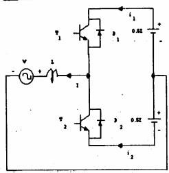
Figure 1: Single-Phase Converter
