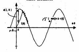
Figure 3: Typical Phase Modulator Sliding Response
