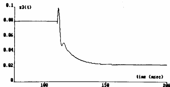
Figure 3. Output current response to a step change in the set-point value (output current control mode)
