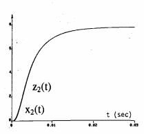
Figure 2(b). Average and Actual Output Capacitor Voltage Response for a Dynamical PWM Stabilization of Full Bridge Buck Converter.
