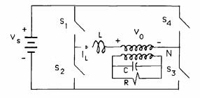
Figure 1. Full Bridge Buck Converter
