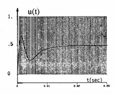
Figure 2(a). Average and Actual Input Inductor Current Response for a Dynamical PWM Stabilization of Full Bridge Buck Converter.
