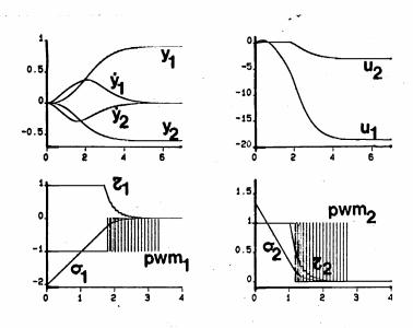
Figure 1. Dynamical PWM controlled response of two-degree-of-freedom robotic manipulator.
