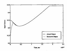
Figure 1: Response of the actual and estimated average normalized inductor current
