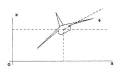
Figure 1: Planar Vertical Take-Off and Landing Aircraft System.
