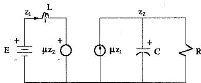
Figure 1: Equivalent circuit of the average PWM model of the “boost” converter circuit.
