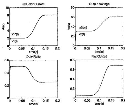
Figure 2: Simulation of state feedback controlled “boost” converter.
