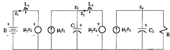
Figure 3: Equivalent circuit of the average PWM model of the “boost-boost” converter circuit.
