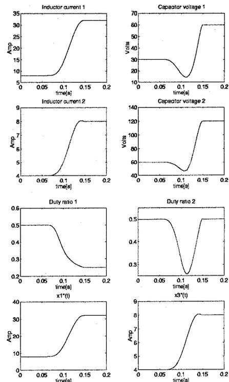
Figure 4: Simulation of state feedback controlled “boost-boost” converter.
