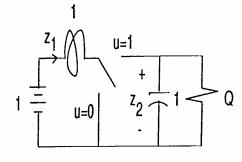
Figure 1: Normalized "boost" converter circuit
